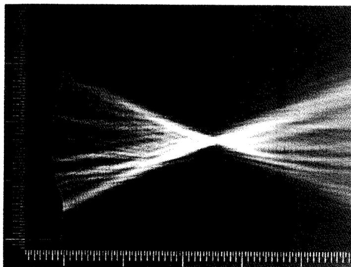
Figure 4. Schlieren image of CW acoustic beam.
