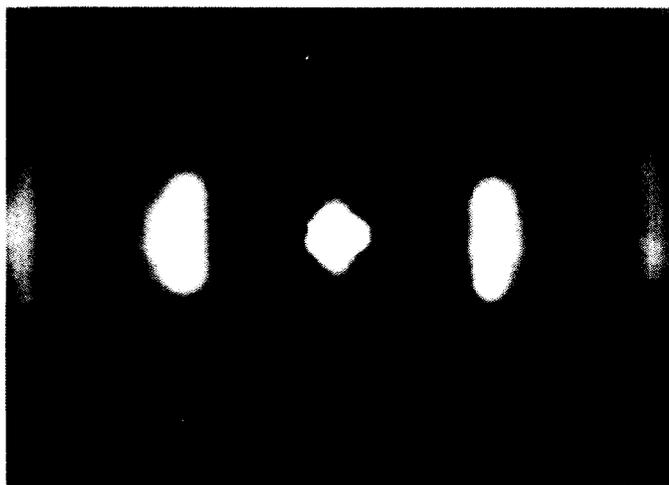
Figure 2. Diffraction pattern at the focal plane (near field). Zero-th order is at the center, first orders and second orders appear at each side.
