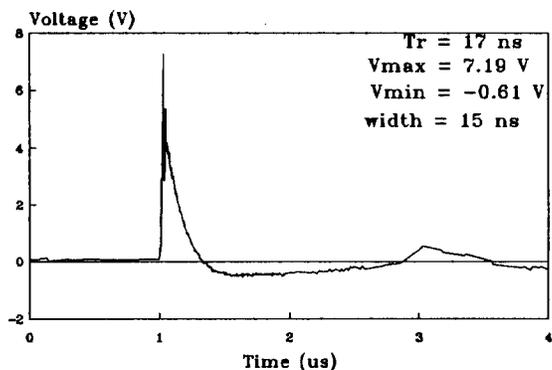
Fig. 1(a) - Shock wave as measured with a Marconi coplanar 1 mm membrane hydrophone.
