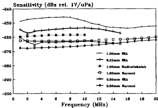
Fig. 7 - Hydrophone sensitivities when loaded by an equivalent impedance of  $1M\Omega$  in parallel with  $30pF$ .
