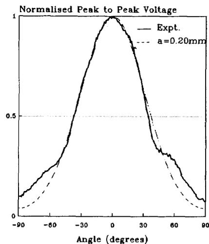
Fig. 6 - Angular response of a 0.25 mm spot poled ceramic hydrophone at 4 MHz.
