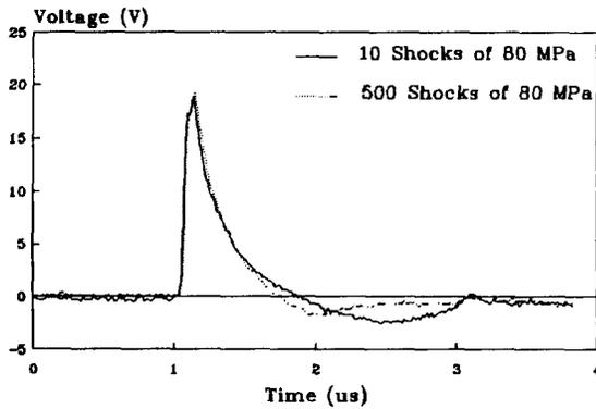
Fig. 2 - Pressure measurement at the focus of a piezoelectric lithotripter before and after 500 shocks of 80 MPa.
