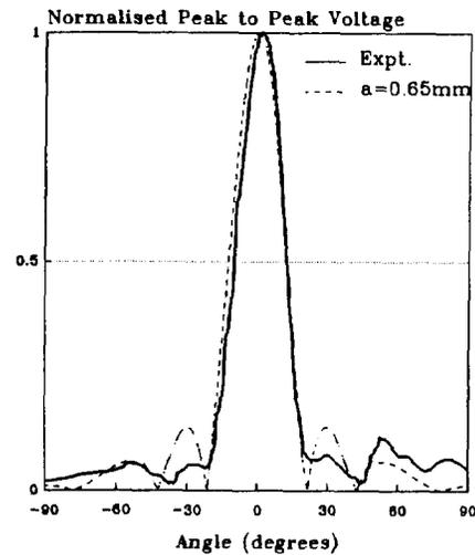
Fig. 3 - Angular response of a 1 mm spot poled ceramic hydrophone at 4 MHz.
