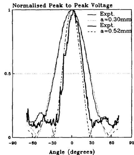
Fig. 4 - Angular response of a 1 mm coplanar and 0.5 mm bilaminate Marconi hydrophone at 4 MHz.
