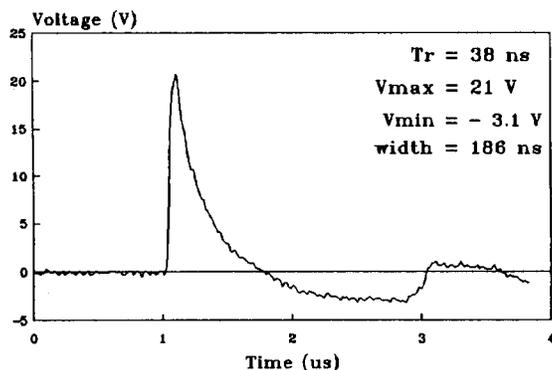
Fig. 1(b) - Same shock wave measured with a 15 MHz, 1 mm spot poled ceramic hydrophone
