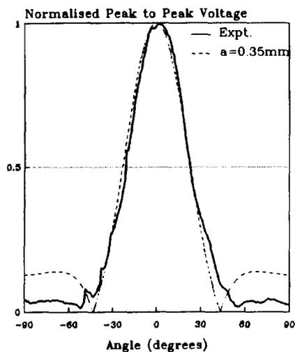
Fig. 5 - Angular response of a 0.5 mm spot poled ceramic hydrophone at 4 MHz.
