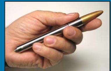
AG-2010 preamplifier with HGL-0200 hydrophone
